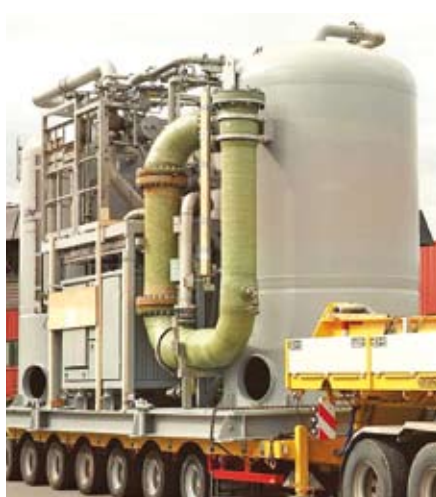
The pictures above show one of the two water treatment packages which Jotne designed, manufactured and tested. The packages are now in place on the Bonga platform off the coast of West Africa.
