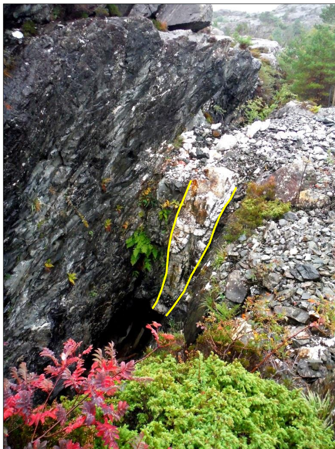
Figure 3-7 Quartz vein (c. 60 cm wide, between the yellow lines) in the Haugesundsgang workings, possibly left as a pillar to support the hanging wall. View towards the southeast (SRK ES, 2018)
