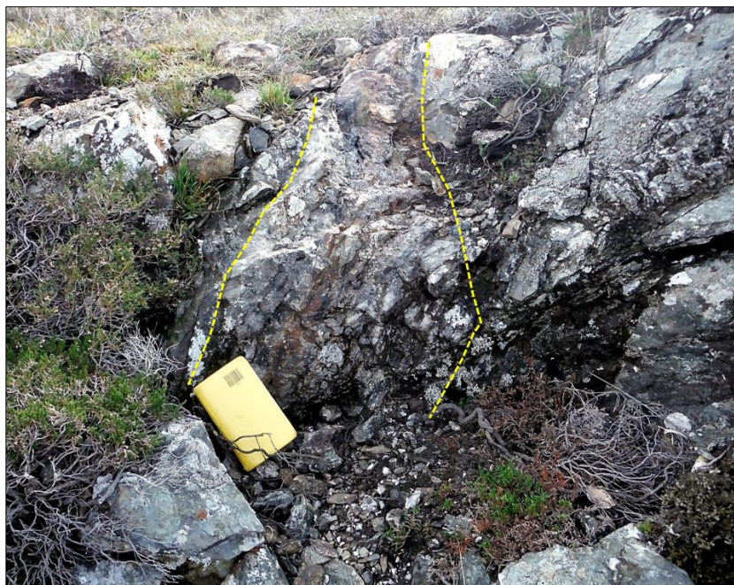
Figure 3-16 Outcrop of gold-mineralised quartz-sulphide vein in sheared gabbros in the southern part of the licence (SRK ES, 2018)
