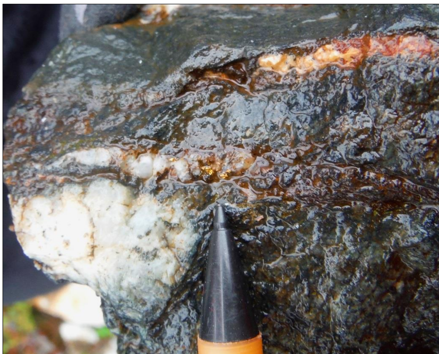
Figure 3-19 Coarse gold observed in gabbroic rocks with quartz stringers at the Modums-Gravene workings (SRK ES, 2018)
